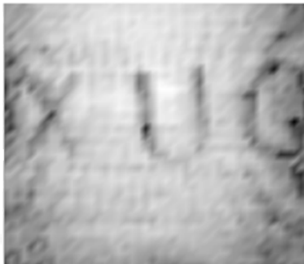
Figure 22b: The amplitude reconstruction of the letters 'XUO' without padding operation
