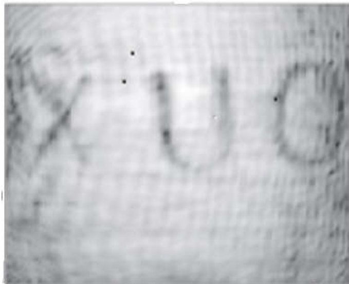
Figure 21b: Amplitude reconstruction of the letters 'XUO' after zero padding operation.
