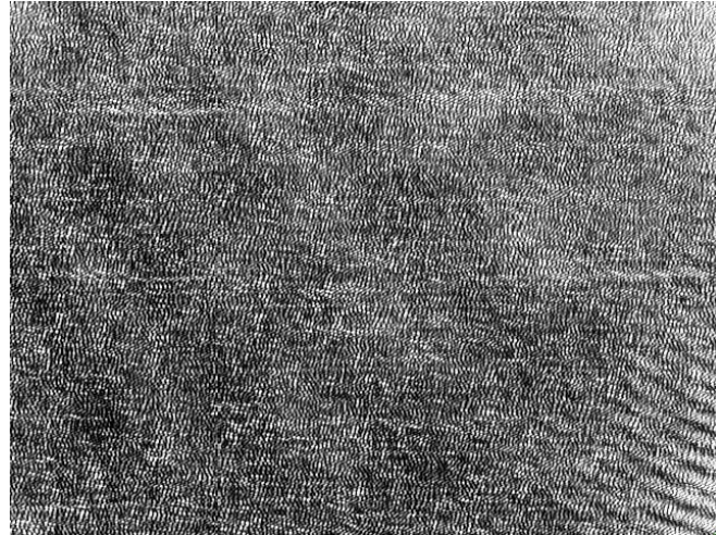
Figure 20a: The interferogram recorded from the aluminium block with ‘ROU’ inscription.
