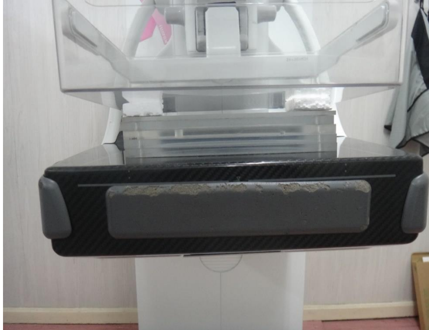
Figure 21: Set – up for Image quality test on 45 mm phantom with spacer to obtain an equivalent breast thickness of 53 mm
