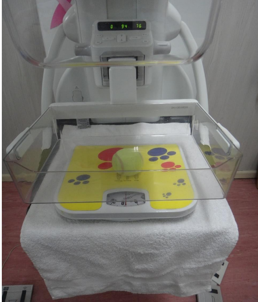
Figure 17: Set – up for measuring Compression force in both Automatic and Manual Mode
