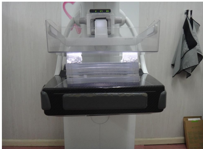
Figure 22: Set – up for Image quality test on 70 mm phantom with spacer to obtain an equivalent breast thickness of 90 mm
