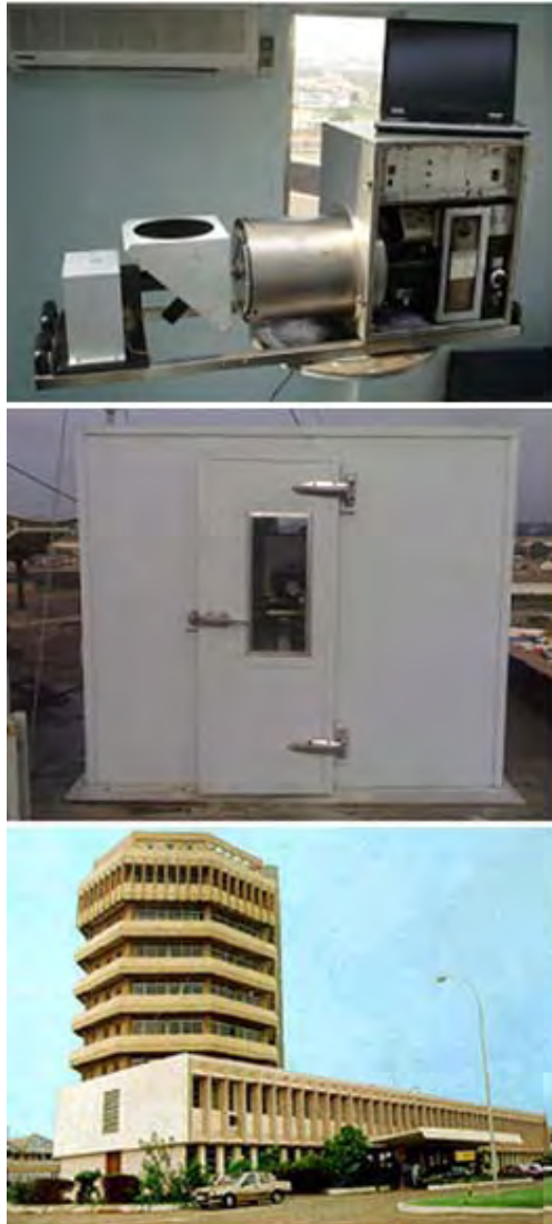
Plate 6: Top picture - The DOAS system as it was mounted within the housing
