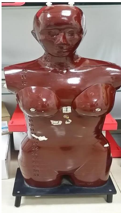
Figure 4: Picture of Rando (female) anthropomorphic phantom sectioned transversely for dosimetric studies.
