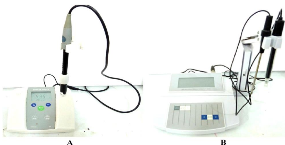
Figure 19: (A) Bench Top pH Meter (FE20-ATC Kit, USA) (B) Microprocessor Conductivity Meter (ODS 120W, India)
