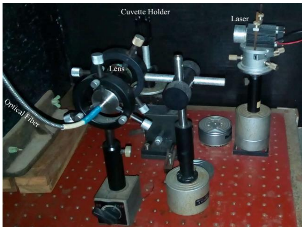
Figure 22: Laser Induced Fluorescence Experimental Set Up Made Up of a Diode Laser, Lens and Lens Holder, Cuvette Holder, Optical Fibre (Partly Shown), Filter (Not Shown), a USB 2000 Spectrometer (Ocean Optics, USA) (Not Shown), and a Del Computer (Not Shown).
