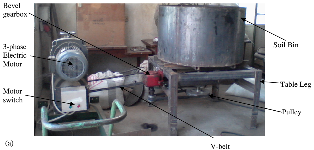
Fig. 2: A 3-dimensional view of the soil bin showing (a) bin support frame, (b) circular soil bin, (c) the assembly drawing
