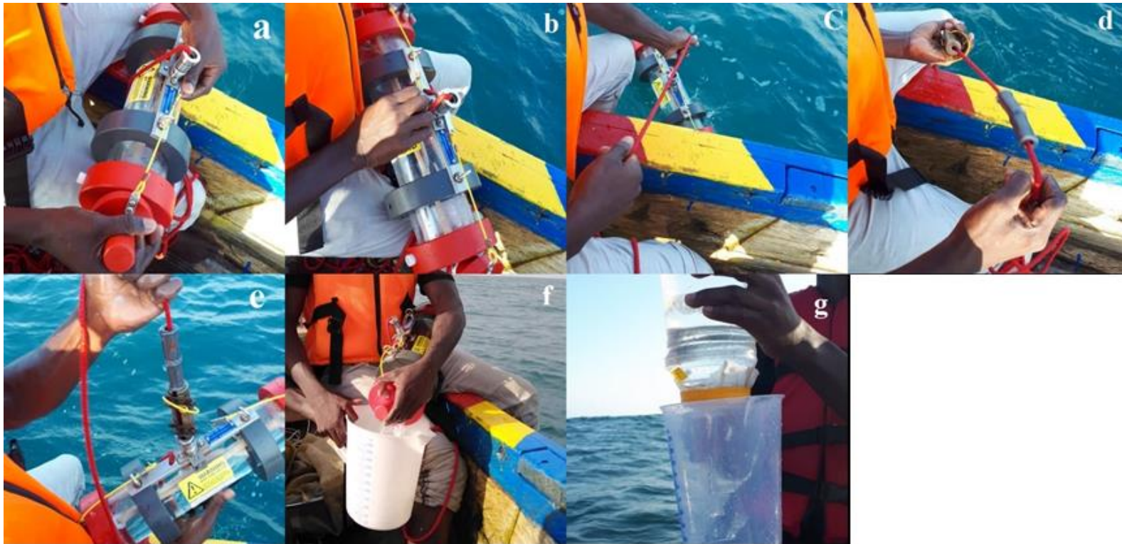
Figure 3. 3: Procedure for the vertical sampling of marine copepod; (a-b) corking and (c) lowering of water sampler, (d) releasing messenger, (e) drawing, (f) emptying sampler and (g) filtering sampled water.
