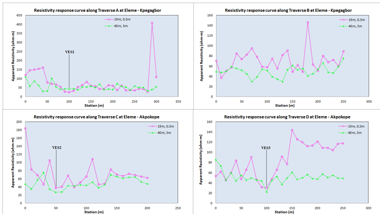
Figure 4: Resistivity Response Curve of Traverses at Eleme-Kpegagbor.
