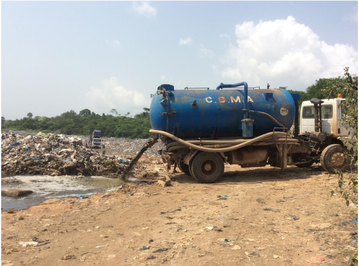
Figure 3: A truck releases faecal sludge into the environment in Nkanfoa (source: Investigations by the authors)
