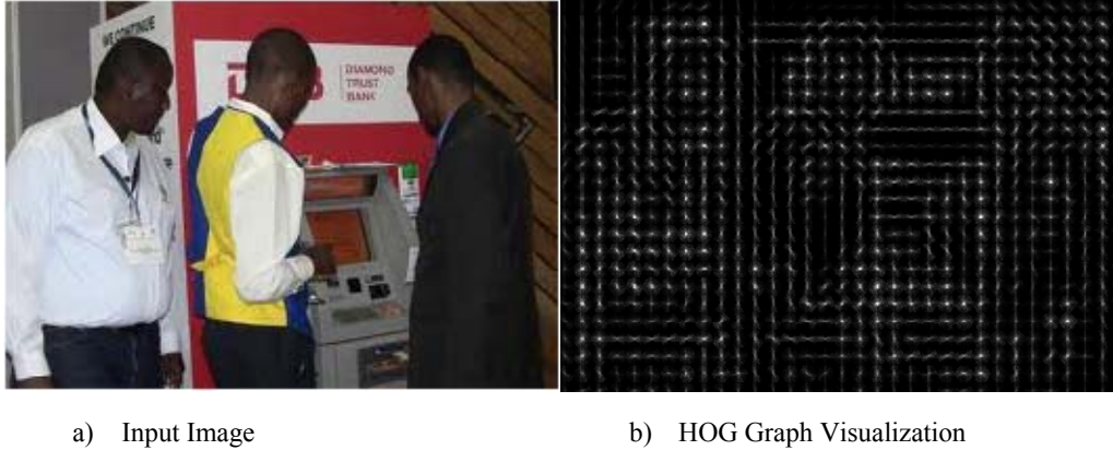
Fig. 4: (a) Input RGB image and (b) Visualization graph of the Histogram of Orientated (HOG) descriptors of the input image.
