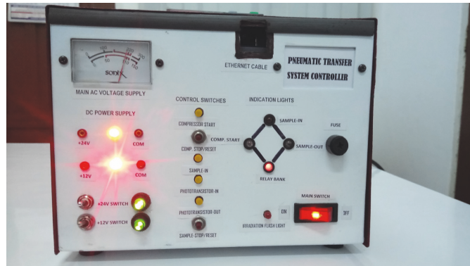
(a) Front view of the pts controller unit
