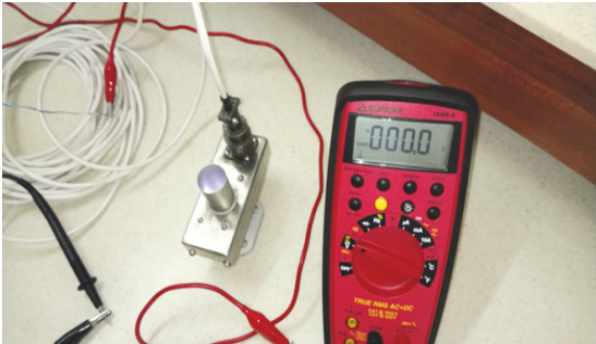
FIGURE 19: Illumination of led in sample slot phototransistor outputs 0.00 volts.
