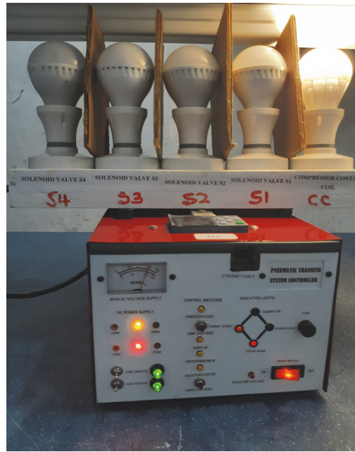
FIGURE 14: Contactor coil energized, compressor starts.
