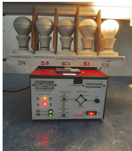
FIGURE 17: Solenoid valves S1 and S3 close, sample irradiation starts with flash light/beeps of buzzer.
