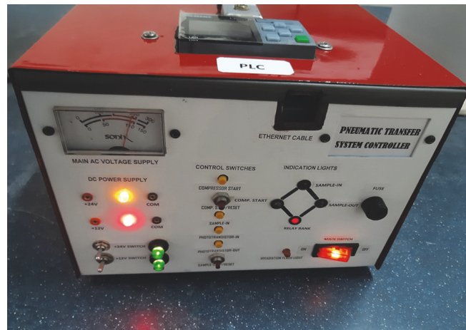
(b) PTS controller unit showing the PLC
