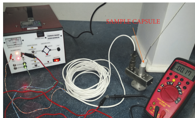
FIGURE 18: Sample capsule moved out of detection and phototransistor outputs 0.00 volts.
