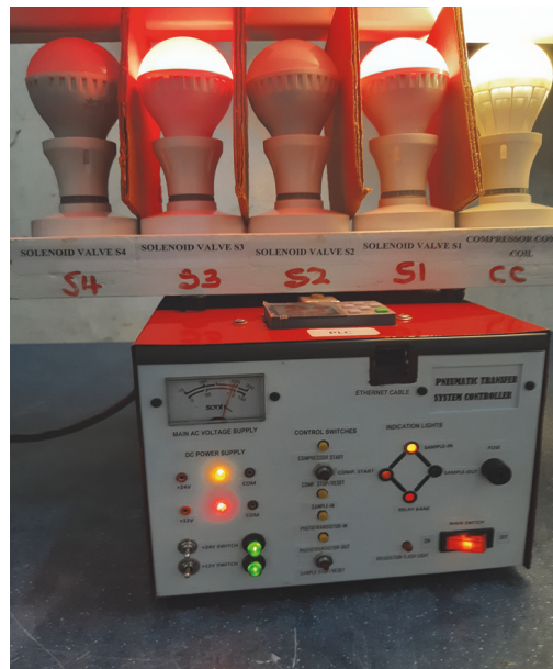
FIGURE 15: Sample-in button depressed, solenoid valves (S1 and S3) open.
