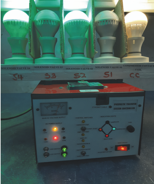
FIGURE 20: Irradiated sample transferred onto detection for counting. Solenoid valves S2 and S4 open.
