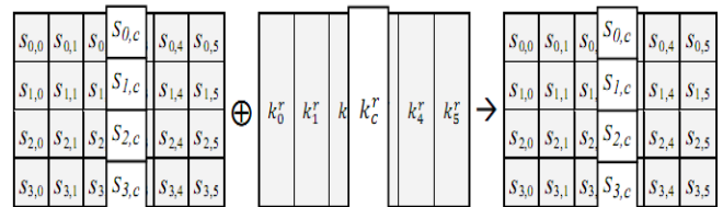
Figure 6. Words from the key schedule are XOR'd into columns in the state.
