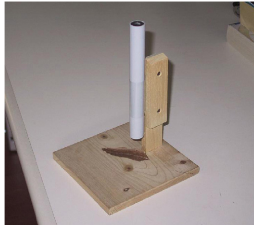
Figure 4. Essential microscope set-up with two recovered lenses from single-use disposable cameras. The object is a dry leaf. Illumination is from ambient light.
