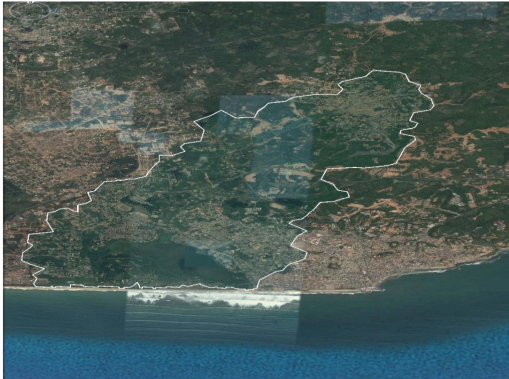
Figure 4.41: Watershed delineation using USGS Earth Explorer (geodataset April 2018)
