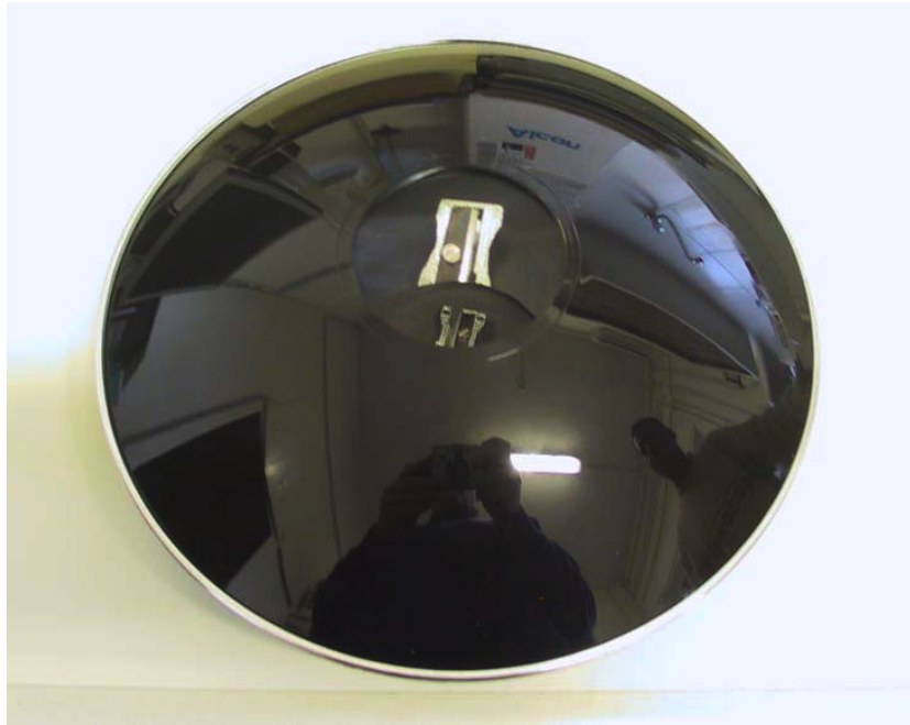
Figure 2. Two-mirror imaging of a simple object (pencil sharpener). The image is at the top and the object at the bottom.
