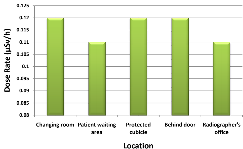
Figure 2. Variation of Dose Rate against Location for X-ray using 77 \text{ KeV} and 20 \text{ mAs} .
