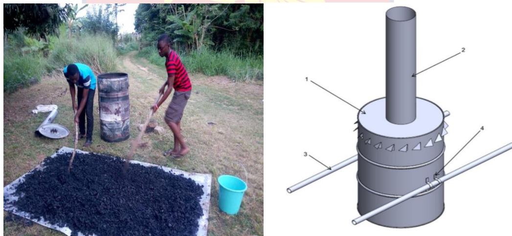
Figure 3: Drying of pineapple waste biochar and the Elsa barrel used to produce the biochar
