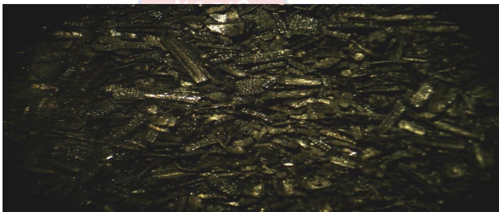
Figure 11: Microstructure of rice husk ash (RHA) used as an amendment
