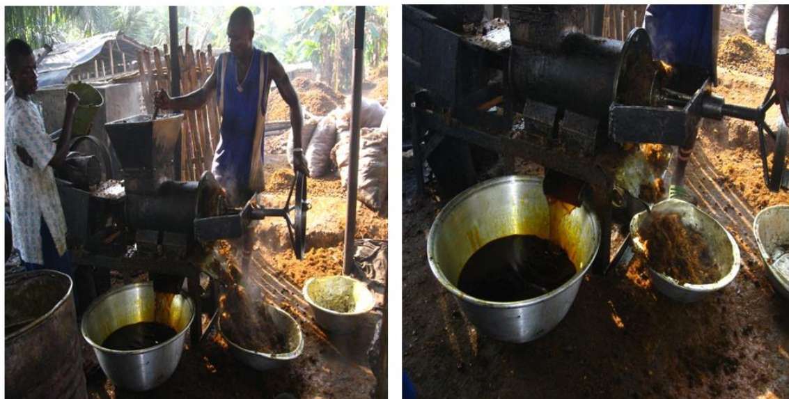
Plate 2. Extraction stage of the processing of palm oil by small-scale palm oil producers (Source: Fieldwork, 2011)
