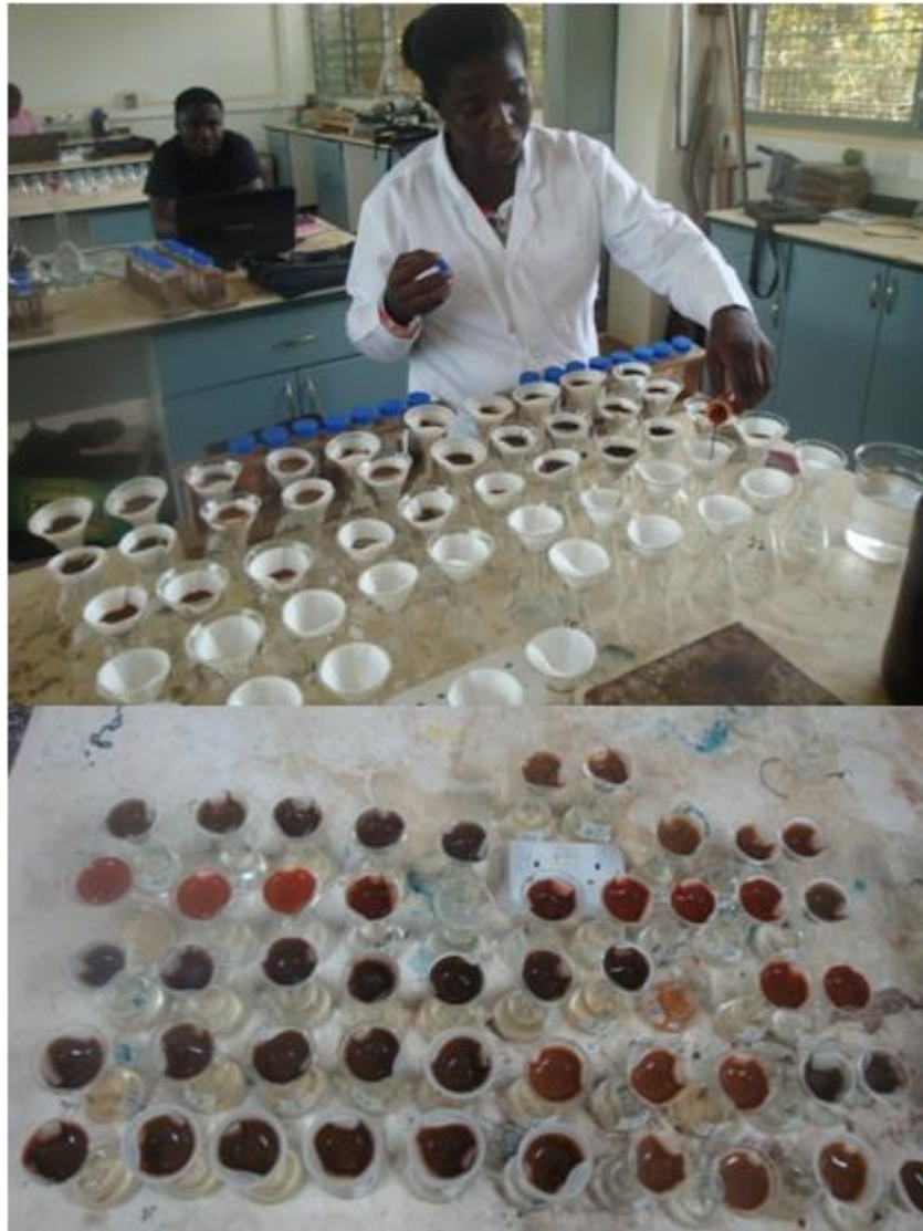
Figure 7: Extraction of micronutrients from soil for Atomic Absorption Spectroscopy (AAS) analysis
